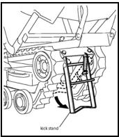
Turn the Key to "Off", unlock the Handle and fold the Power Evacu-Trac closed by squeezing the pair of red Release Levers located underneath, below the Operating Controls.
