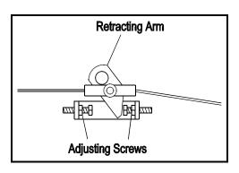
3. The final step is to ensure that the Track Parking Brake is functioning correctly. It is designed to stop and hold rated load on the stairway. To do this, the Brake Spring must pull on the Brake Mechanism without any resistance from the Brake Cable. This can happen if the Front Brake Cable does not have sufficient slack.
