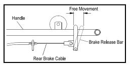
When you squeeze the Brake Release Bar it should travel until it just makes contact with the lime green Handle. This will allow you to comfortably hold Brake Release Bar in its released position when pushing Evacu-Trac on flat surfaces or descending a stairway.
