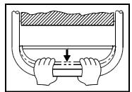
8. At landings, push down on the Handle and turn Evacu-Trac with all the weight on the Rear Auxiliary Wheels. Keep to the inside of the corner for maximum turning clearance. Align the machine at a right angle to the stairs and proceed down the next flight.
