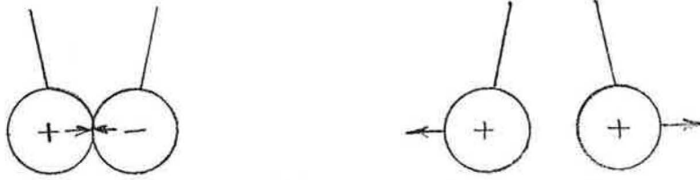
11-1. ELECTROSTATIC FORCES. (a) ATTRACTION OF UNLIKE CHARGES. (b) REPULSION OF LIKE CHARGES. (PHOTO)
